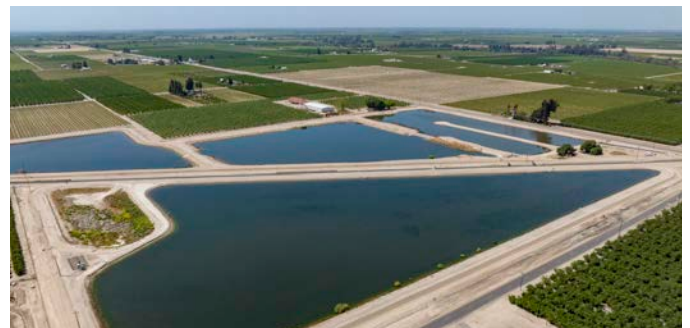
Groundwater recharge ponds, like this one near Fresno, help recharge underground aquifers with surplus water from storms in 2023.
